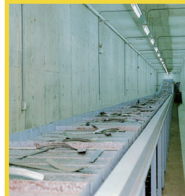
裙板式廢料輸送機 An application example of apron conveyor system for waste materials.
