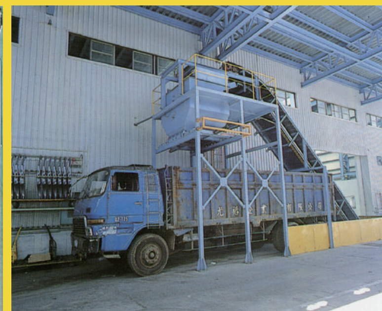
儲料筒具自動卸料功能，方便卡車載運。 The storage tauh features automatic release for convenient loading on a truck.
